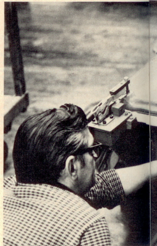
Above. A quality control inspector in the forming department at Piper Aircraft's Lock Haven, Pa., plant inspects a just-formed acrylic transparency that will become the windshield of a Super Cub. Sitting at about a pilot's distance from the transparency, the inspector checks for distortion and light transmittance, as well as for visible blemishes and scratches. Like this windshield, those of most general aviation aircraft are formed by simply draping a heated, cut-to-size acrylic sheet over a mold and letting it cool.
