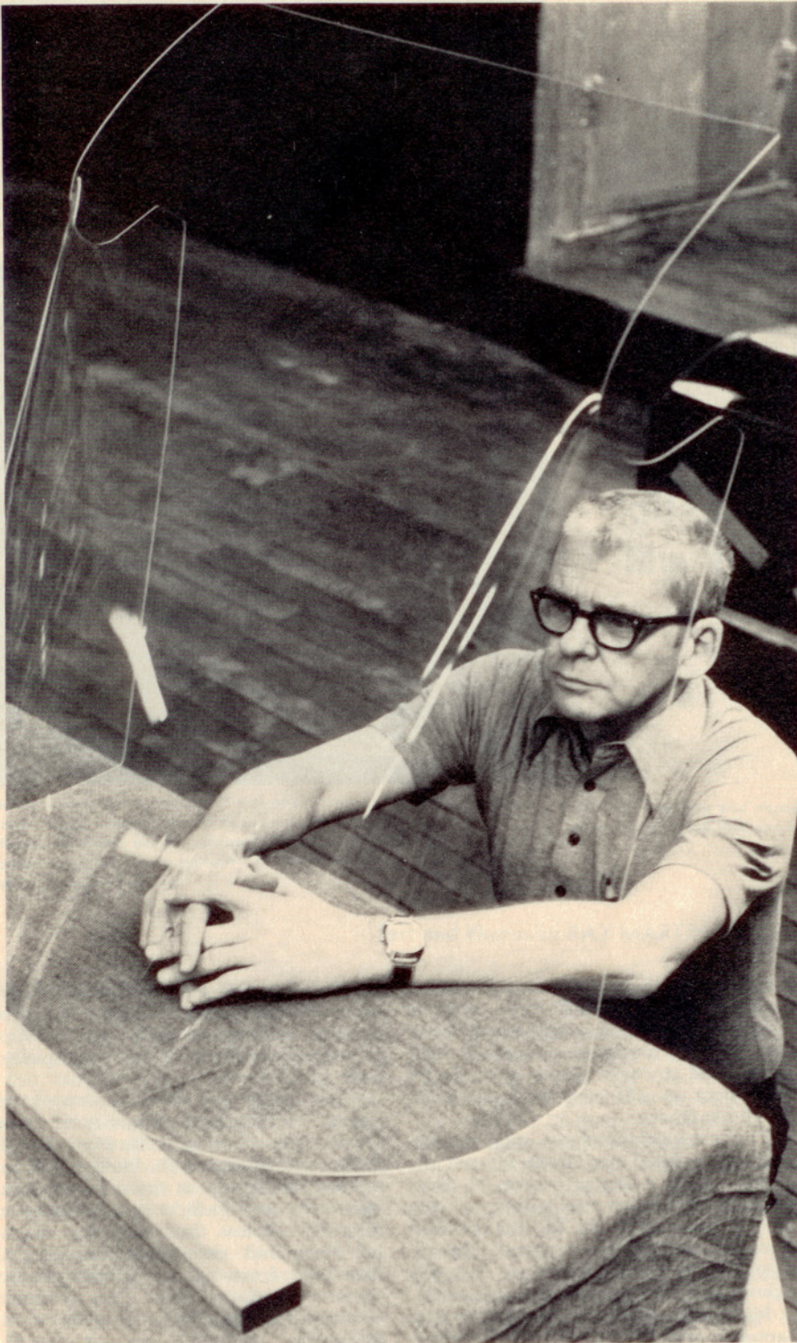
Above. A quality control inspector in the forming department at Piper Aircraft's Lock Haven, Pa., plant inspects a just-formed acrylic transparency that will become the windshield of a Super Cub. Sitting at about a pilot's distance from the transparency, the inspector checks for distortion and light transmittance, as well as for visible blemishes and scratches. Like this windshield, those of most general aviation aircraft are formed by simply draping a heated, cut-to-size acrylic sheet over a mold and letting it cool.
